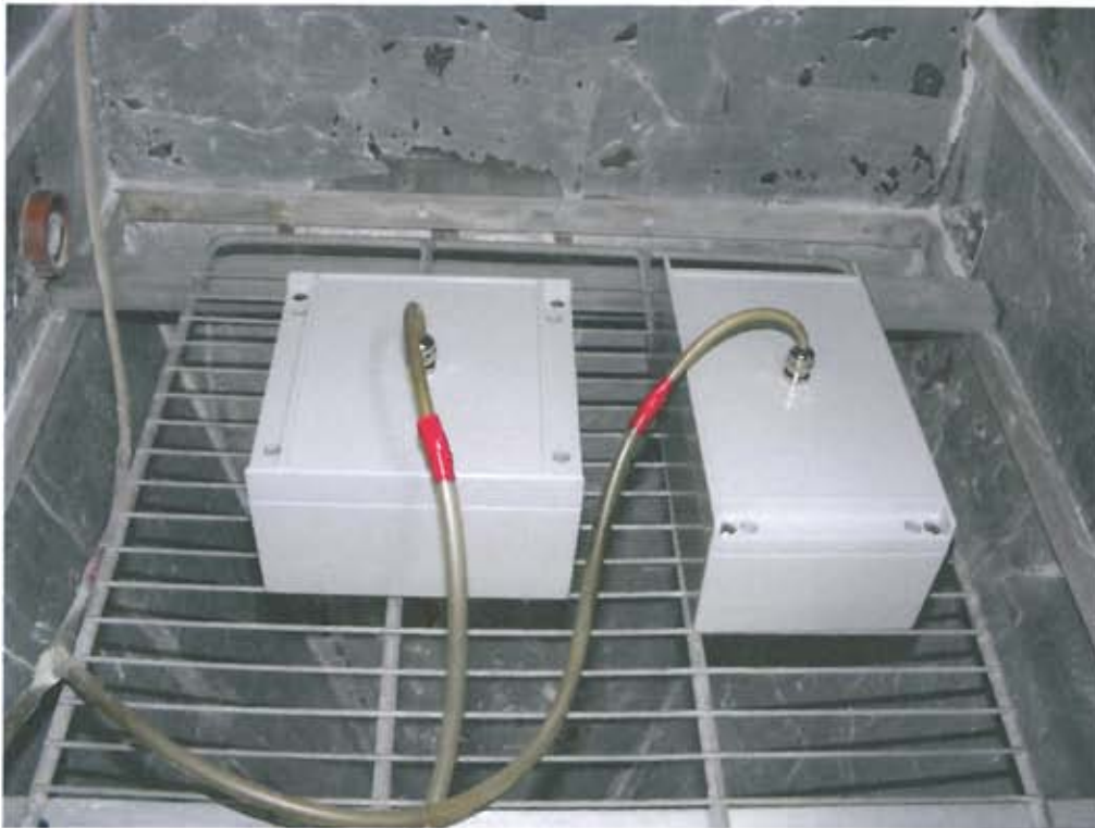
Figure 2 loading of dust, IP Code 6X, second run
