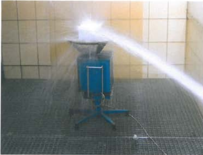
Figure 3 IP Code X6, loading by strong jet of water, exemplarily
