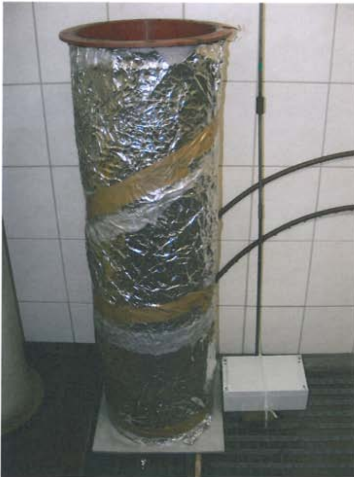
Figure 4 IP Code X7, loading by dipping, exemplarily
