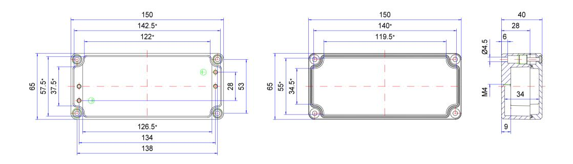
\* Please note: Mould slope for casting ejection, dimensions in the amount of the bottom!
