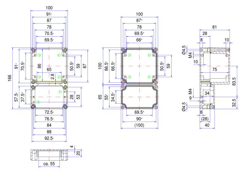
\* Please note: Mould slope for casting ejection, dimensions in the amount of the bottom!
