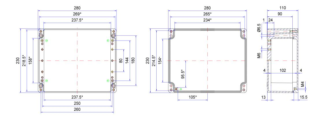
\* Please note: Mould slope for casting ejection, dimensions in the amount of the bottom!
