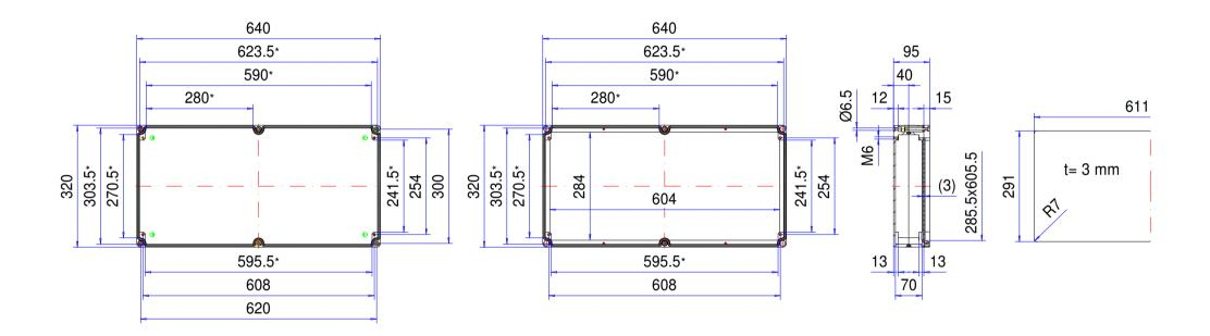
\* Please note: Mould slope for casting ejection, dimensions in the amount of the bottom!
