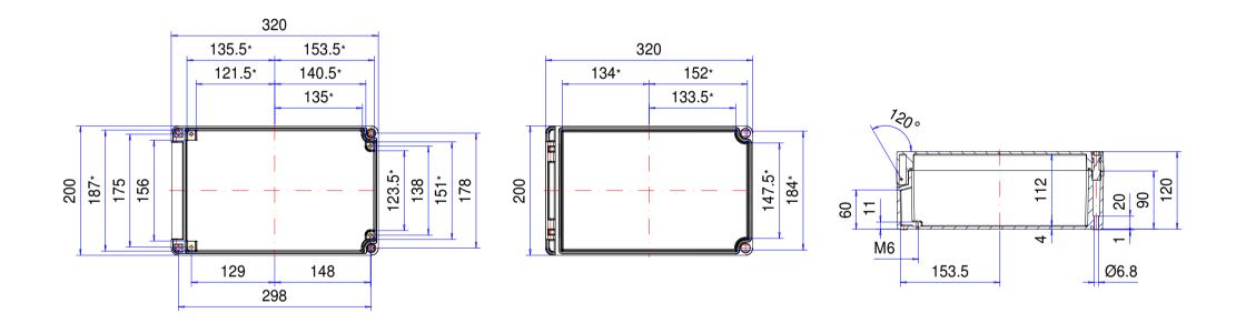
\* Please note: Mould slope for casting ejection, dimensions in the amount of the bottom!
