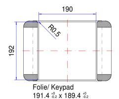
\* Please note: Mould slope for casting ejection, dimensions in the amount of the bottom !
