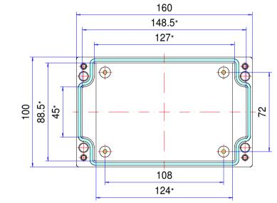
\* Please note: Mould slope for casting ejection, dimensions in the amount of the bottom!
