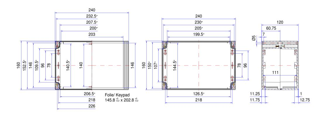
\* Please note: Mould slope for casting ejection, dimensions in the amount of the bottom!
