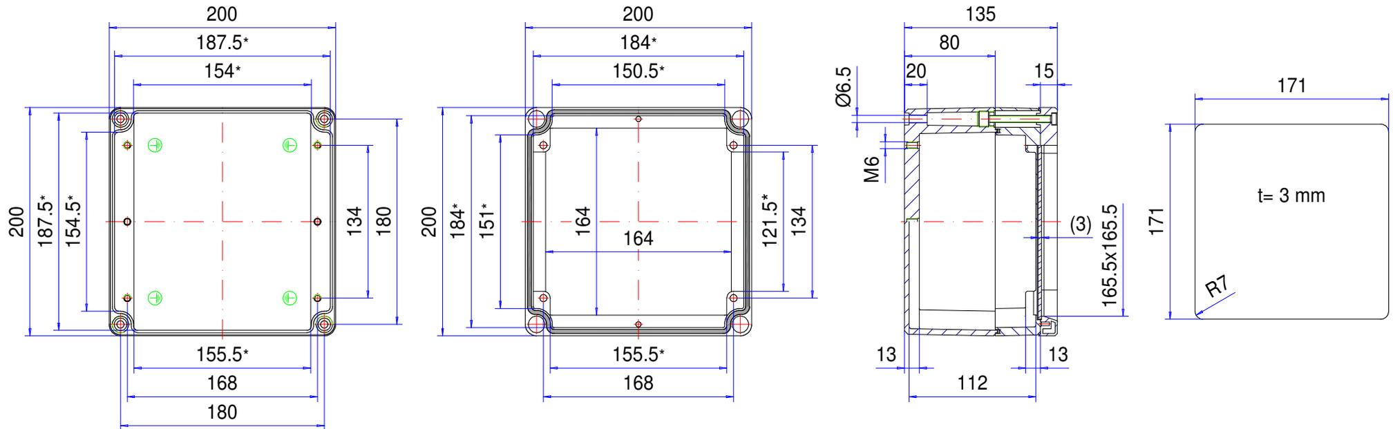
\* Please note: Mould slope for casting ejection, dimensions in the amount of the bottom!
