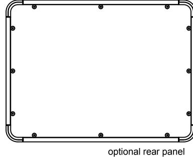
useable front-plate area= nominal size -50 mm area reduction generated by lock and hinge combination
