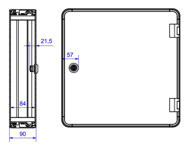
useable front-plate area= 350x350mm area reduction generated by lock and hinge combination
