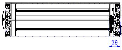
useable front-plate area = nominal size -50 mm area reduction generated by lock and hinge combination
