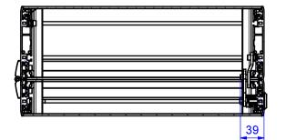
Useable front-plate area = nominal size -50 mm Area reduction generated by lock and hinge combination
