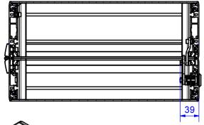
Useable front-plate area = nominal size -50 mm Area reduction generated by lock and hinge combination
