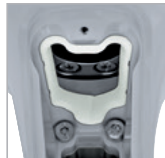
Standard: Integrated cable protection in all joint parts.
